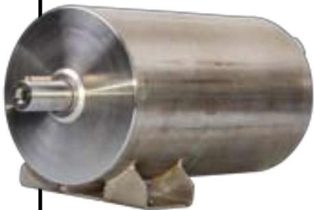
**P**hysically the motors are characterized by a very smooth appearance, which leaves no areas where germs or dirt can collect. The mounting dimensions are according to the IEC72 standard construction forms B5 or B14. Different shaft and / or flange dimensions are available.
